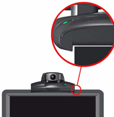
Figure 1-1. Placing the ViewStation
